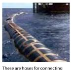
ankers anchored offshore and onshore facilities and transporting crude oil. Since the hoses are installed in the special environment of the ocean, abundant experience and advanced technical capabilities are required for design that fulfills durability requirements in order to withstand severe storms such as typhoons. There are only a very few companies around the world capable of designing and manufacturing marine hoses.
